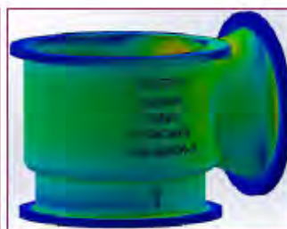
Angular Globe Valve Thermal and Mechanic Analysis
